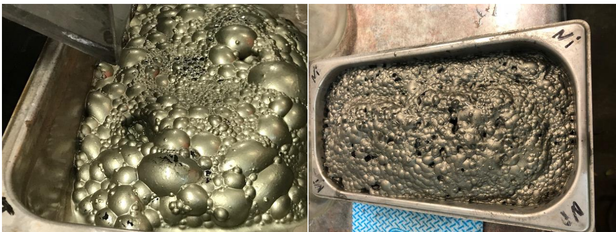
Figure 3. Final copper concentrate (left) and nickel concentrate (right) from Master Composites
