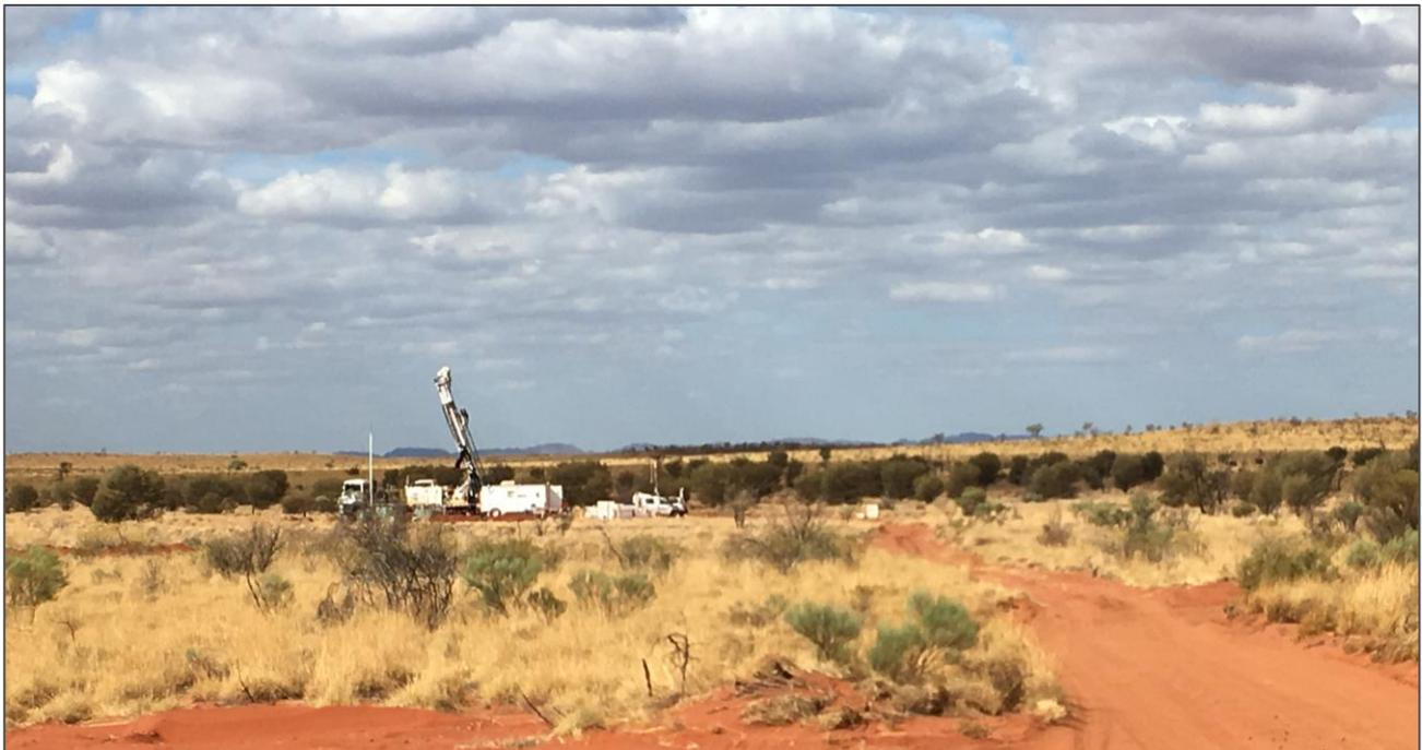
**Figure 3.** Diamond drilling operations at One Tree Hill. Note the extensive sand cover, including sand dunes in the background, which obscures bedrock.
