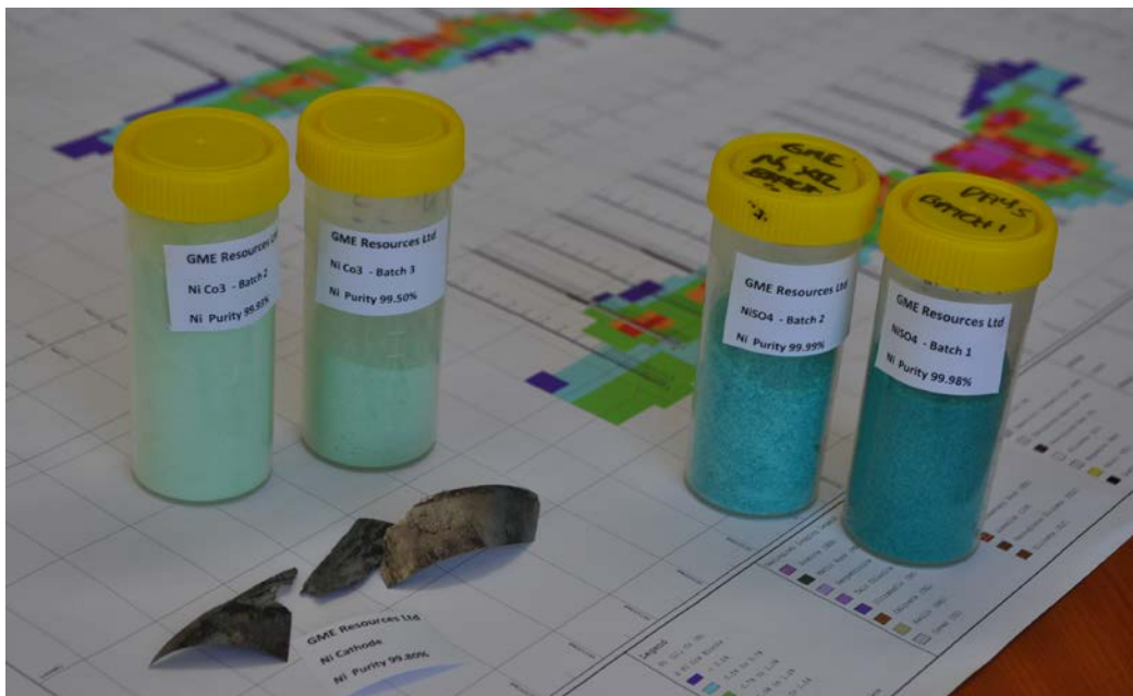
Photo: High purity (+99.95%) Nickel products produced from the NiWest continuous pilot plant.
