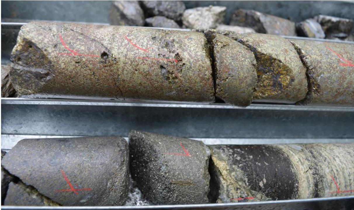
Figure 2 Enlarged image of massive sulphides containing abundant chalcopyrite and sphalerite
