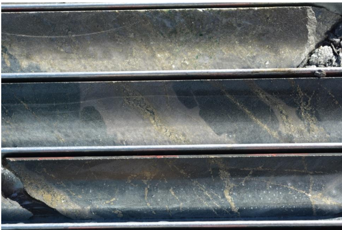
Figure 3 Pyrite stringer veins showing infill and alteration relationships between pyrite and sericite overprinting chlorite in volcanoclastic (389.7m)
