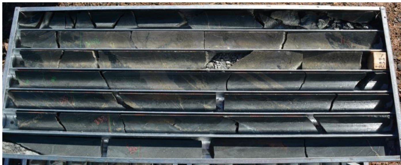
Figure 1 Strongly sericite altered semi-massive sulphide (FOV 386.4 m – 392.8 m)
