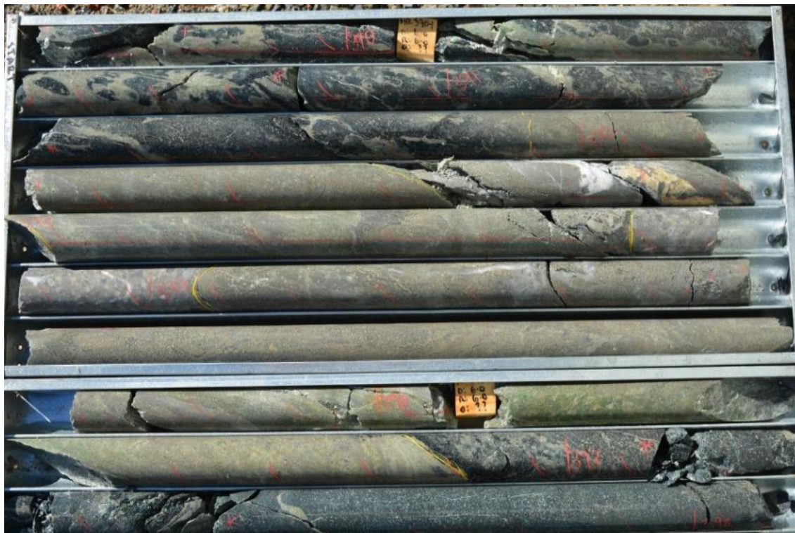
Figure 4 Strongly sericite & pyrite altered intrusive (Andesite) (FOV 389.6 m – 398 m)
