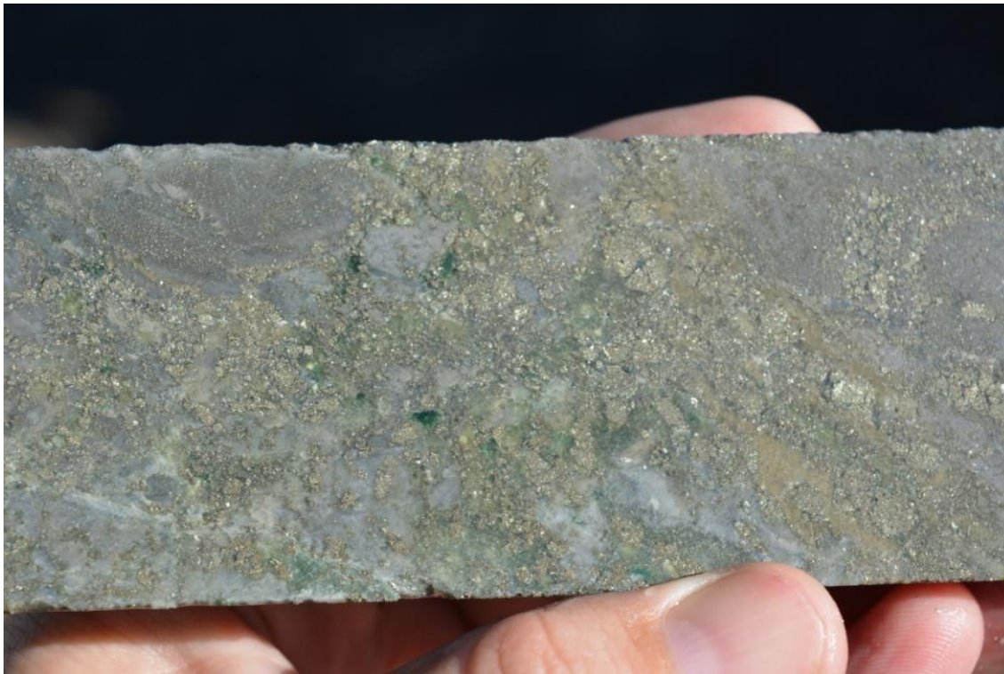
Figure 2 Strongly sericite altered semi-massive sulphide (390.6m)
