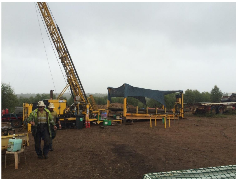
Figure 2 Diamond drill rig at Liantown East (LTED01)
