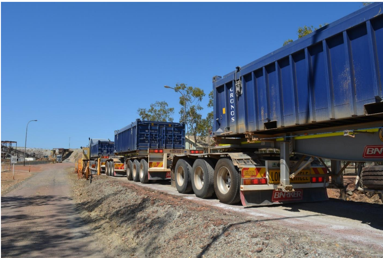
Figure 3 Triple road train being weighed on weighbridge before being loaded
