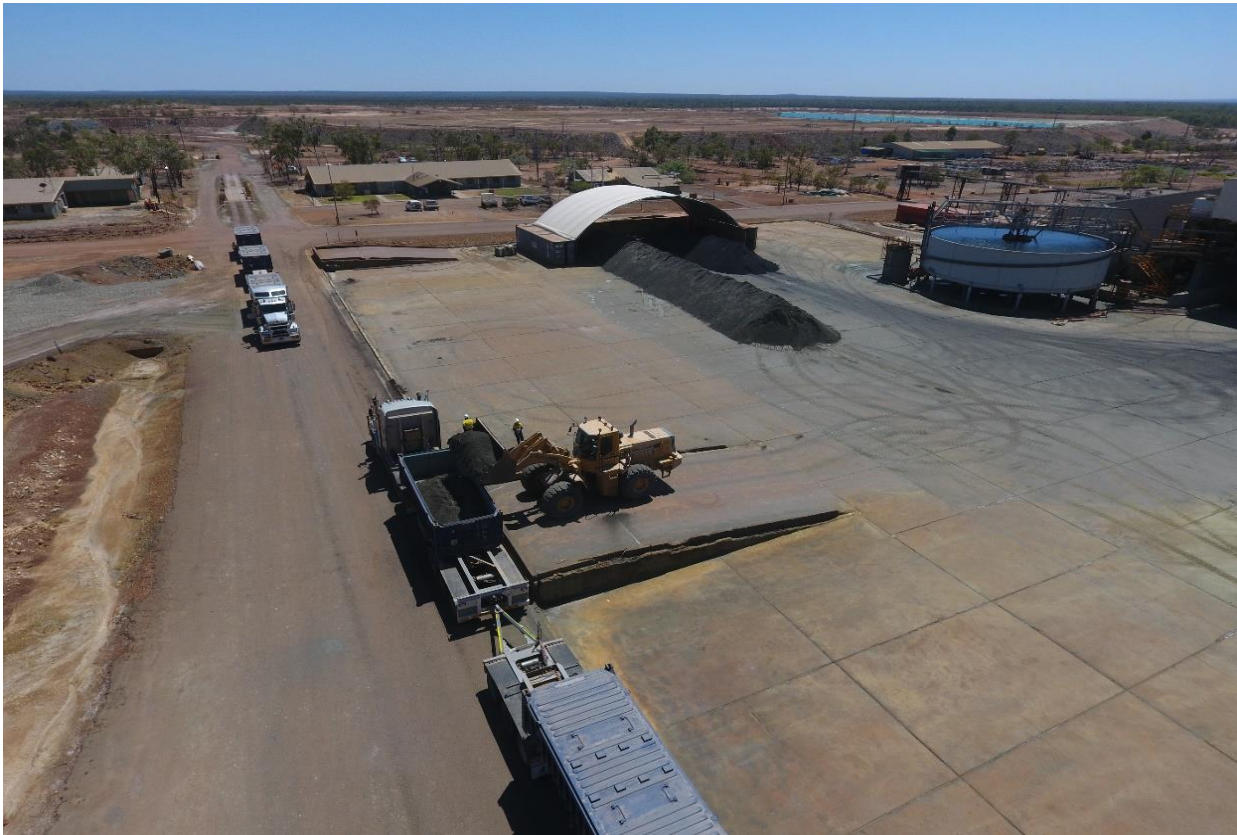
Figure 3 Triple road train being weighed on weighbridge before being loaded
