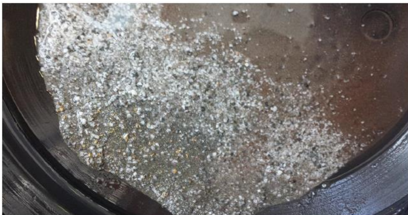
Figure 5 First Stage Knelson Concentrate with abundant coarse visible gold
