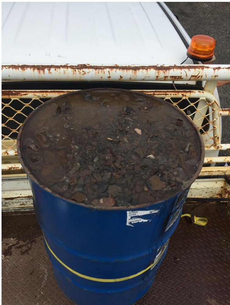
Figure 3 44 gallon drum filled with Bakers Creek Stockpile rock and 94.5L of water.
