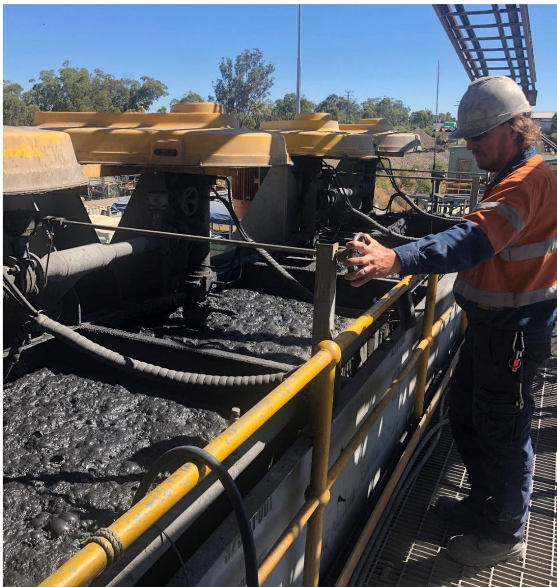
Figure 3 Jameson Cell froth (final gold flotation concentrate)
