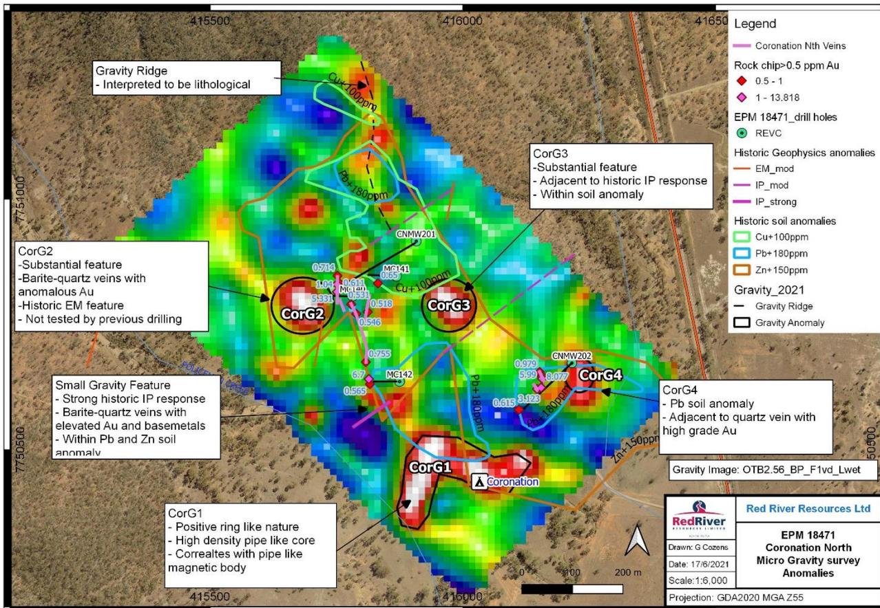
**Figure 2:** Summary plan showing gravity anomalies and associated geochemistry, previous drilling and ground geophysics
