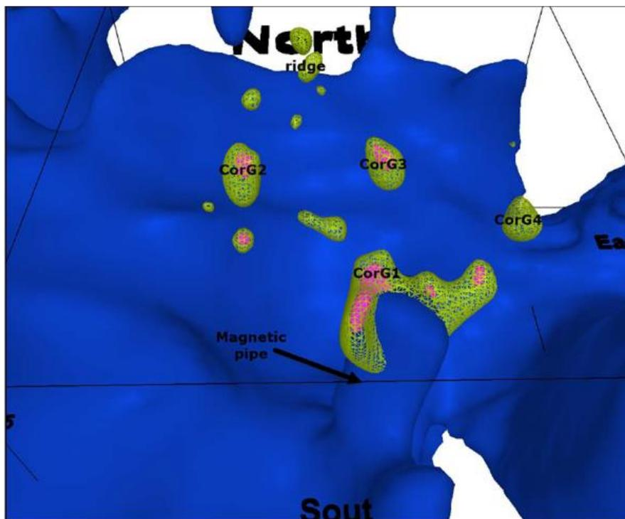
**Figure 3:** 3D Model with gravity anomaly sources
