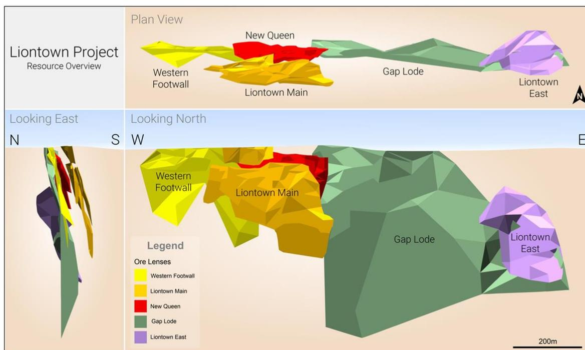
**Figure 1:** Long section of mineralised zones at Liontown
