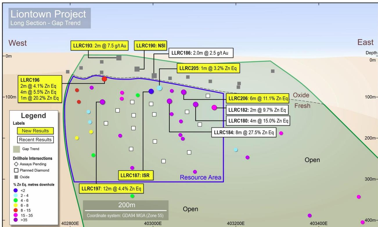
**Figure 2: Gap sulphide infill drilling**
