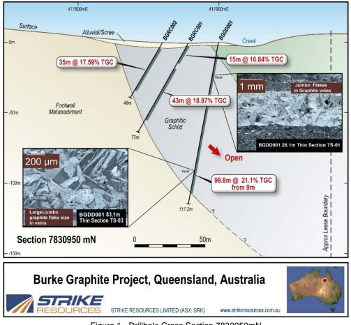
Figure 1 - Drillhole Cross Section 7830950mN
