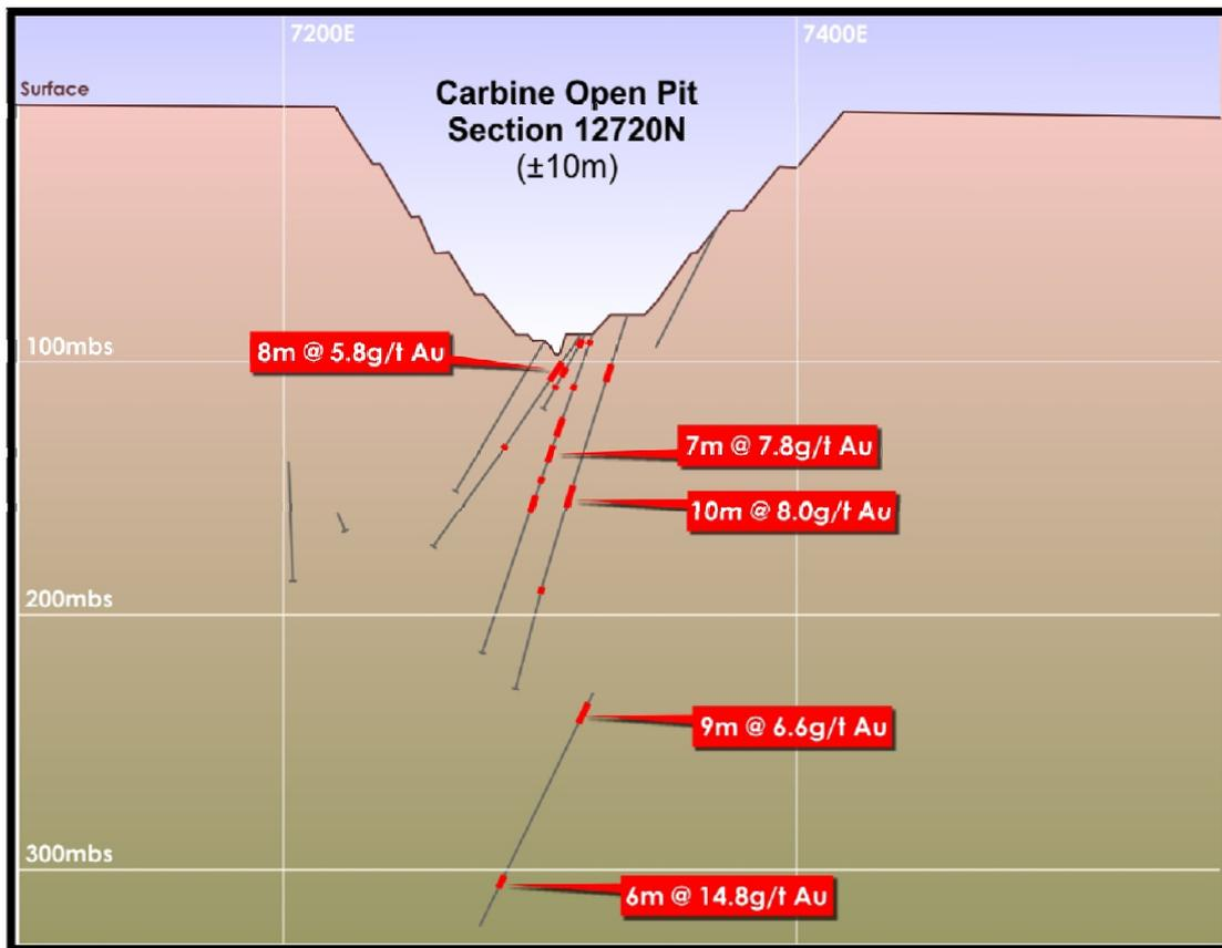
Figure 5 – Carbine Open Pit Cross Section 12720N
