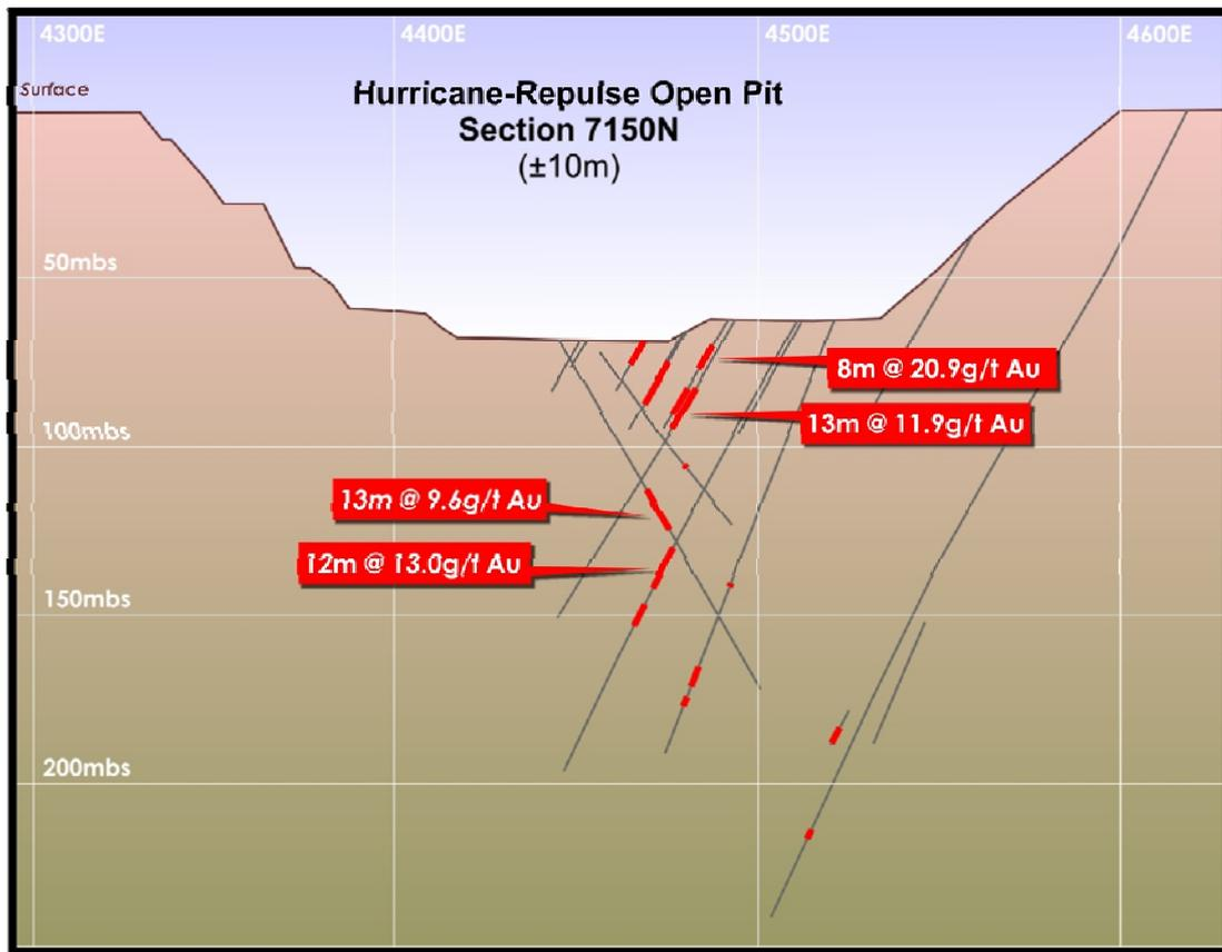
Figure 3 – Hurricane-Repulse Open Pit Cross Section 7150N
