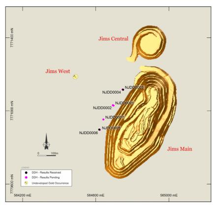
Figure 5 – Plan view of Jims open pits and location of the 2022 diamond drill holes.
