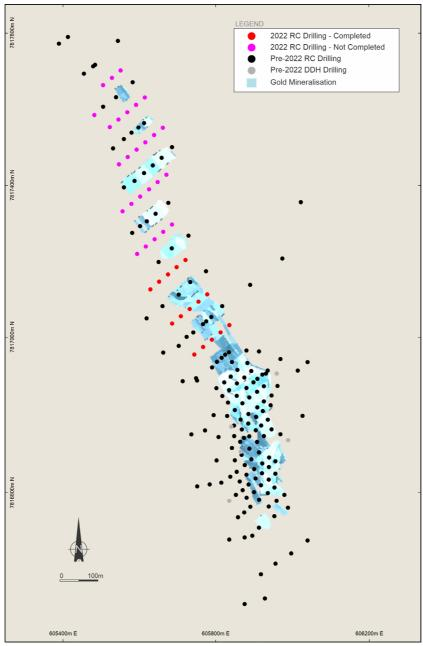
Figure 4 – Plan view of Ripcord and location of drilled and planned drill holes.
