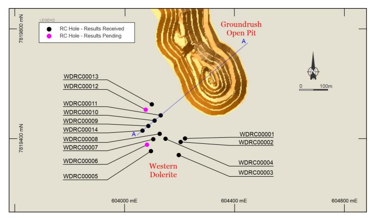
Figure 2 – Plan view of the RC drilling campaign completed at the Western Dolerite Prospect.
