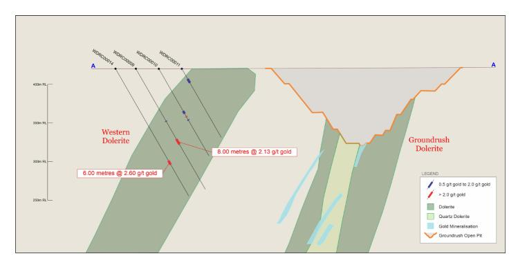
Figure 3 - Western Dolerite Drill Hole Cross Section A-A.
