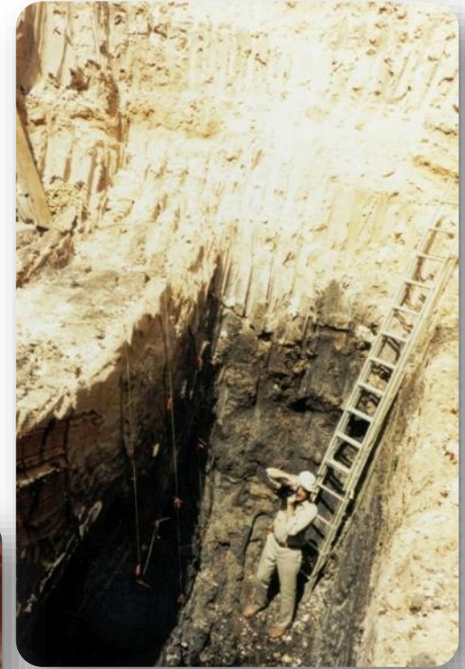
Close-up in Japanese test pit (1980s) showing carbon-rich ore and free dig nature of material
