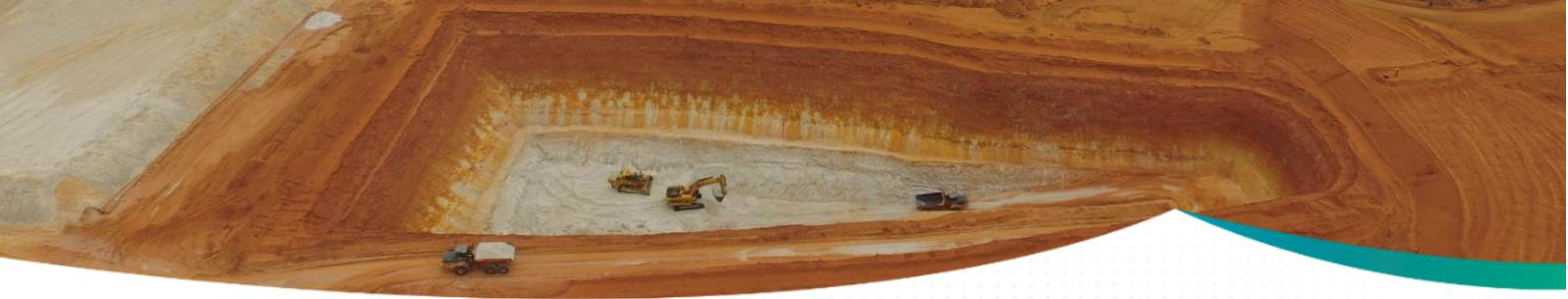
Vimy's proposal of using the mined-out pit voids to create below ground tailings storage facilities, which will be capped and rehabilitated with topsoil and vegetation, provides a safe and permanent tailing storage solution. The Environmental Management Plan for these facilities was approved on 28 August 2020.
