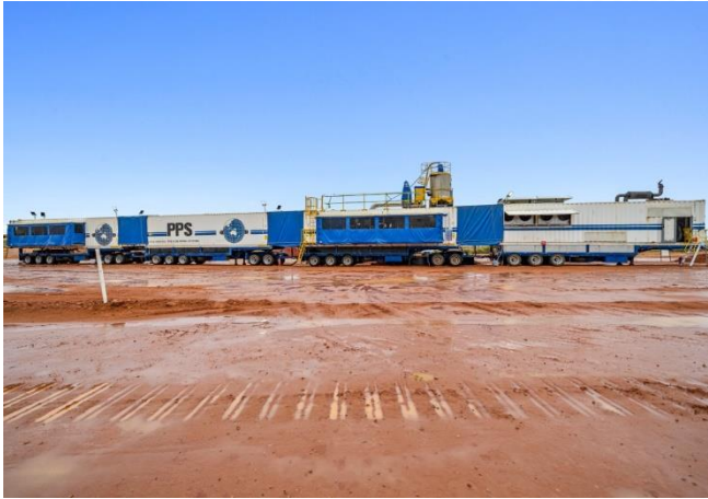
Figure 2 Polyline Pipe Systems pipe extrusion for the raw water borefield
