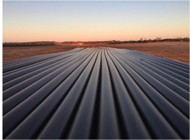
Figure 2 Polyline Pipe Systems pipe extrusion for the raw water borefield
