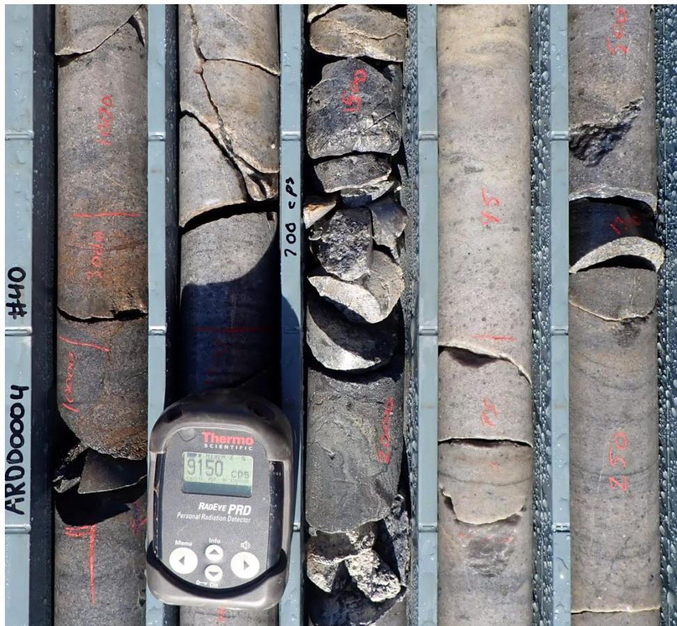
Figure 2: Mineralised faulted Mamadawerre Sandstone in hole ARDD0004 (dosimeter at 222.9m)
