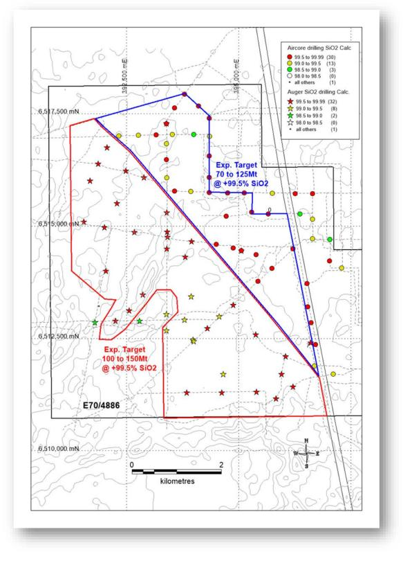
Figure 2: Aircore and auger drilling completed on E70/4886, with exploration targets.
