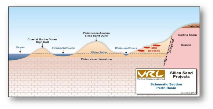
Figure 1. Schematic section of Silica Sand Dune Exploration Target
