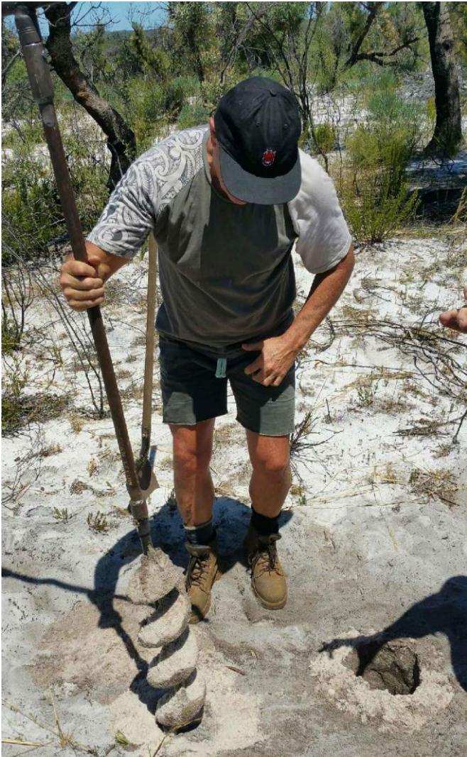
Drilling using 4WD-mounted AC rig and hand held auger
