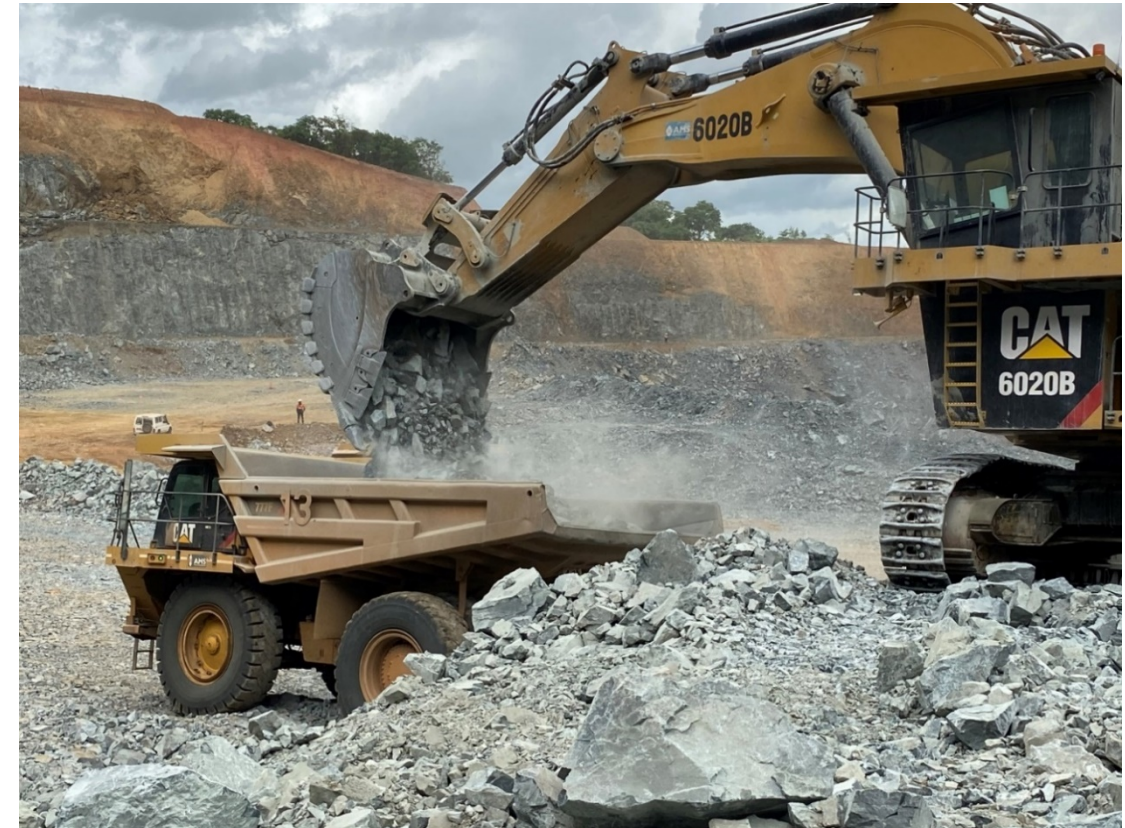
Photo: Recently commissioned Caterpillar 6020B excavator in operation at Mako
