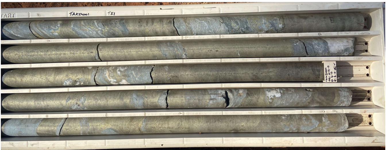
Figure 1 – Core photo from TAKD001 showing the banded massive sulphide intervals between 211.5 metres to 215.8 metres down hole.
