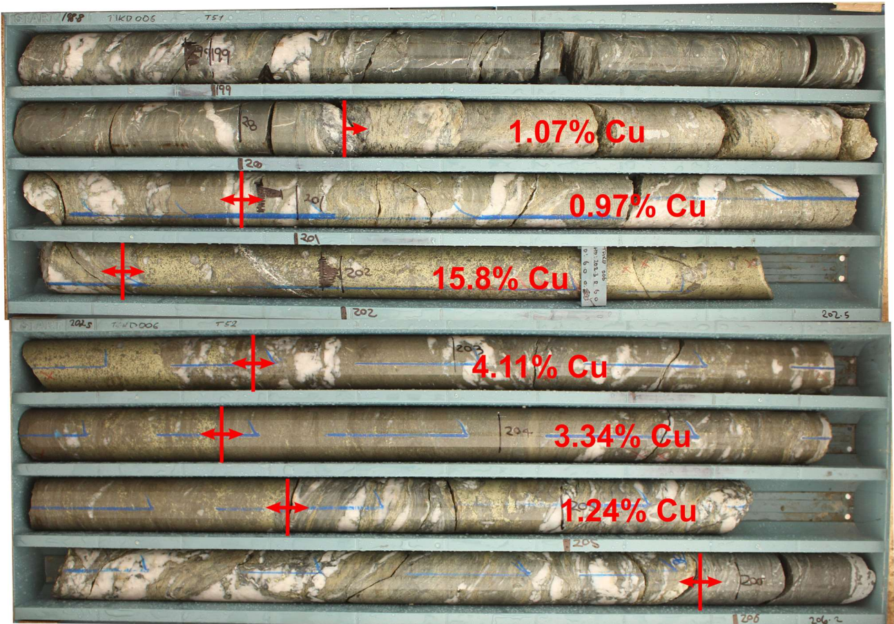
Figure 2 – TAKD006 drill core photo between 198.80 metres to 206.20 metres, highlighting the copper sulphide mineralised interval. Red arrows denote sample intervals and red text denotes Cu assay values.
