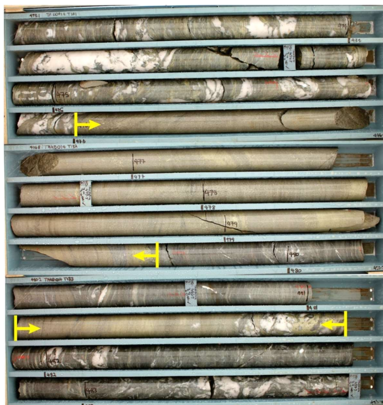
Figure 3 – TAKD014 drill core photo highlighting the massive sulphide mineralised interval between 476.0 metres to 481.9 metres. Yellow arrows denote massive sulphide boundary contacts.
