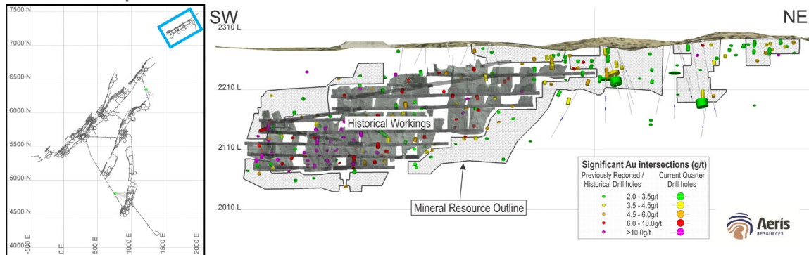
Figure 10 – Long section view showing location of RC drill holes completed during the quarter at the Roses Pride deposit.
