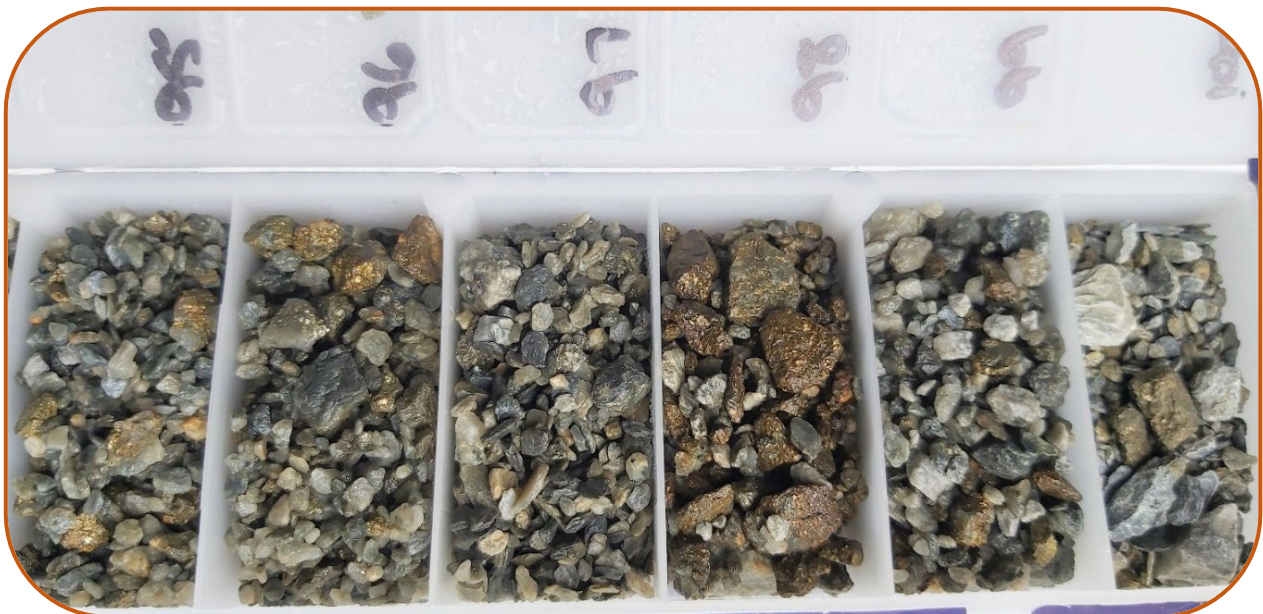
Figure 1: Drill chips from CBLRC023 showing chalcopyrite mineralisation from 94-96 metres with semi-massive pyrite and chalcopyrite from 97-98 metres
