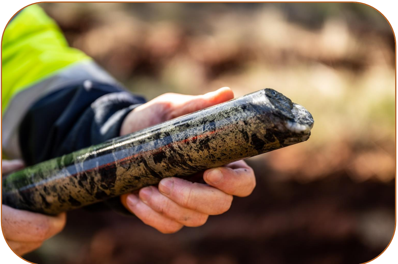
Figure 2: CANDD011, interval of semi-massive chalcopyrite with approximately 20% of chalcopyrite from 152m
