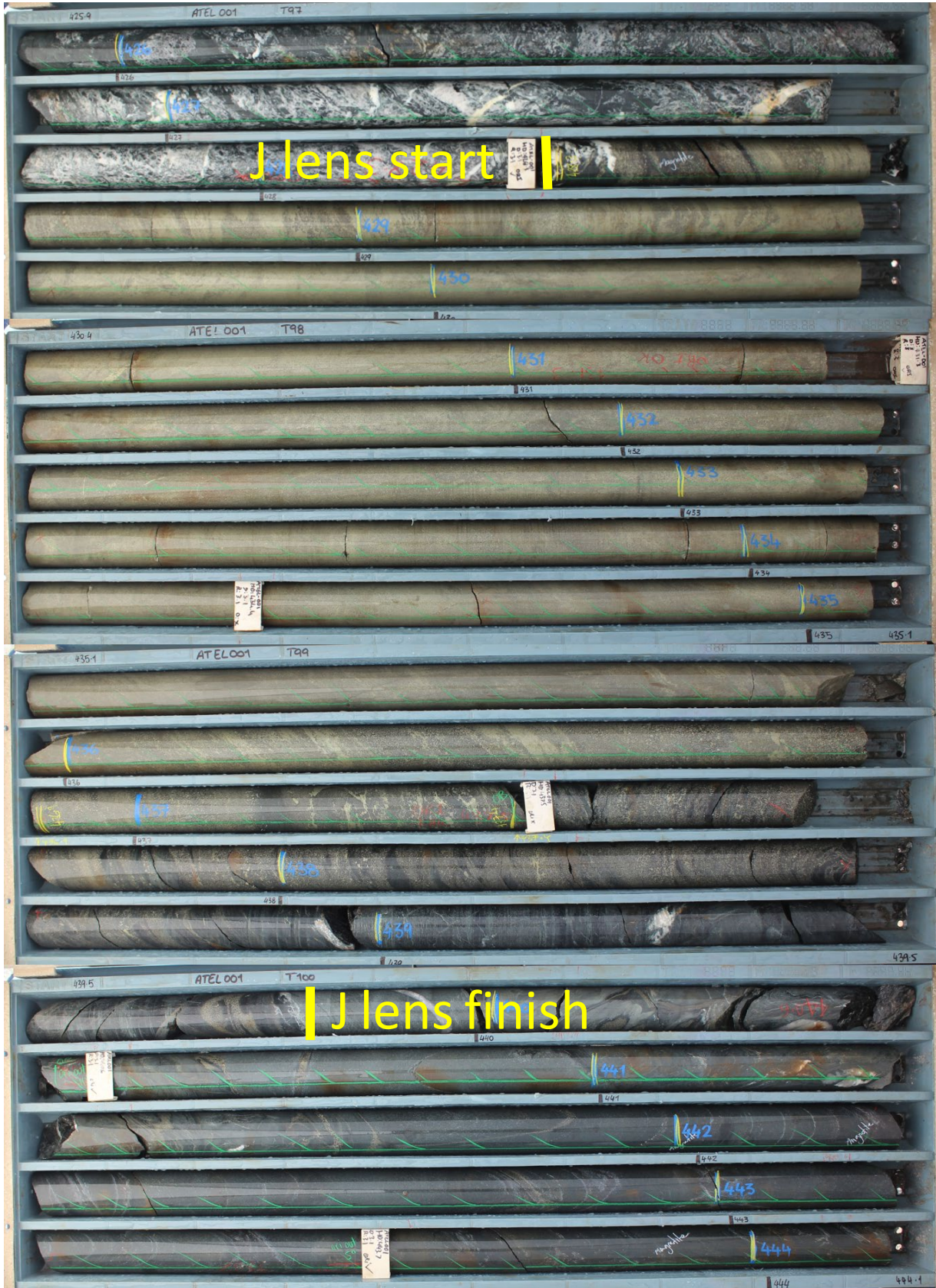
Figure 3 – Core photo from ATEL001 showing a massive sulphide interval through the “J” lens (10.7m @ 5.48% Cu, 0.30g/t Au and 9.7g/t Ag (10.7m true width)).
