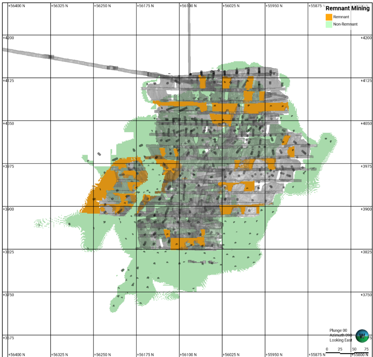
Figure 5 – Long section showing the remnant Mineral Resource for Main Lode and Main Lode Split shown in orange, looking east
