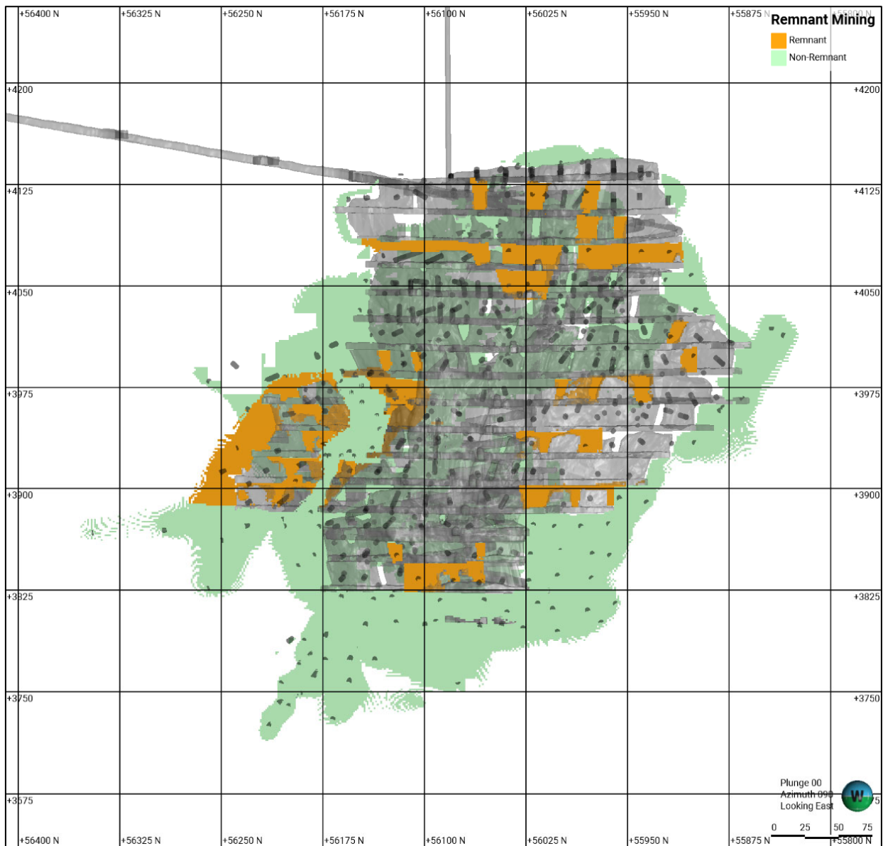
Figure 6 – Long section showing the remnant Mineral Resource for Main Lode and Main Lode Split shown in orange, looking east
