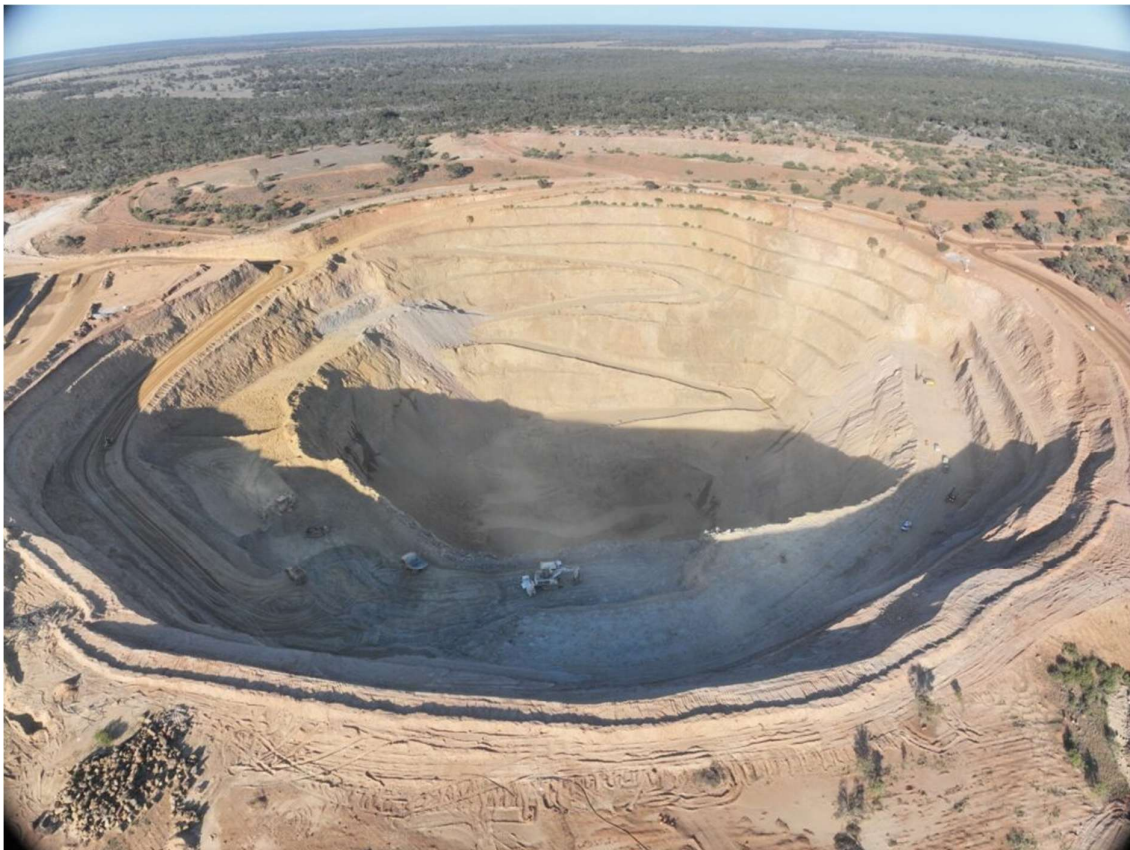
Figure 2: Waste stripping at Murrawombie Pit
