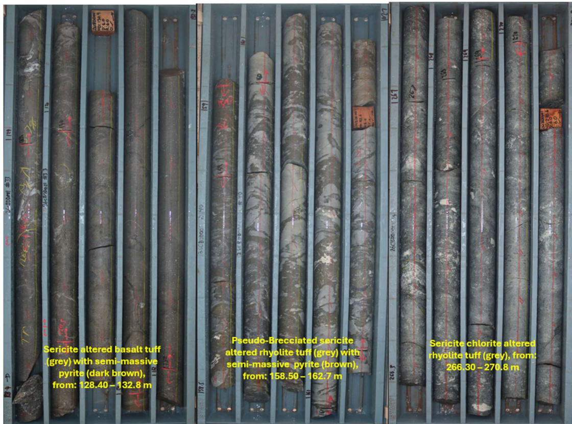
Figure 8: Examples of drill cores from Cerberus prospect hole 26CBDD001. Sericite altered andesite tuff with visual estimates of 3% and up to 10% pyrite (left side); moderate to strong sericite altered pseudo brecciated rhyolite tuff with heavily disseminated pyrite with visual estimates of up to 30% pyrite (brown – dark brown coloured) in places (central); sericite–chlorite altered pseudo brecciated rhyolite lapilli tuff (right)
