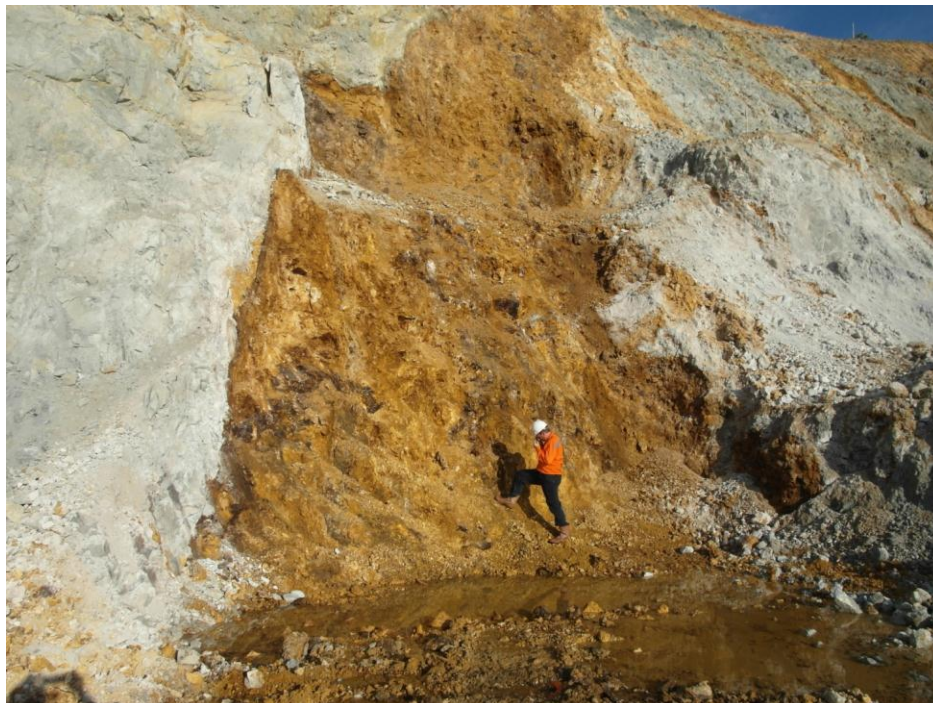
Figure 2. Current exposure of a high grade section of the the Serujan vein in the east wall of the starter pit. The average face grade is 6.2 AuEq (using Ag:Au ratio of 45:1). True width of the vein is approximately 9m.
