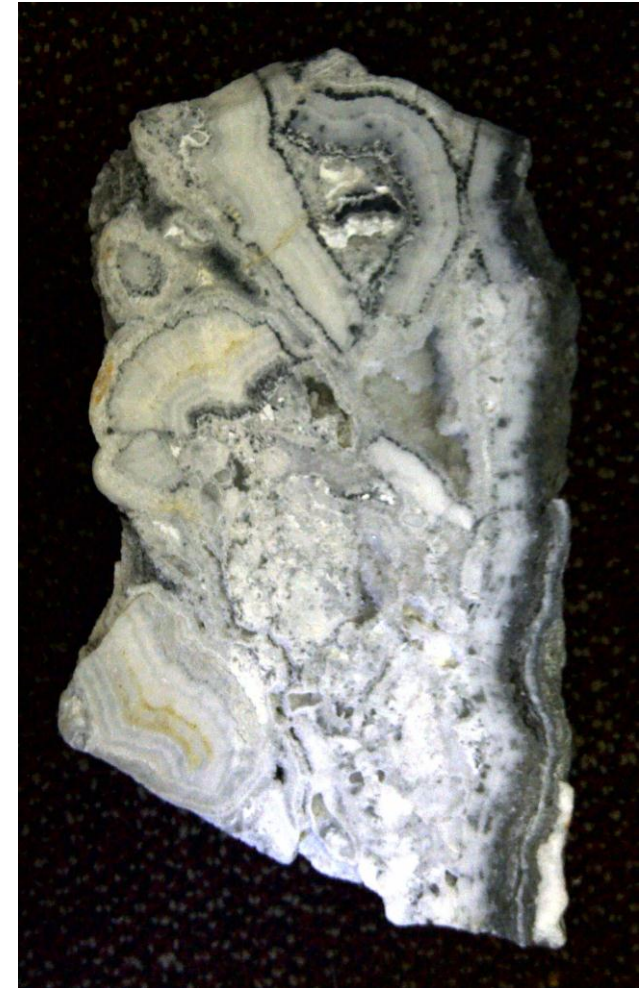
Botol epithermal vein showing coliform structure and black sulphide mineralisation. 125 mm x 75 mm
