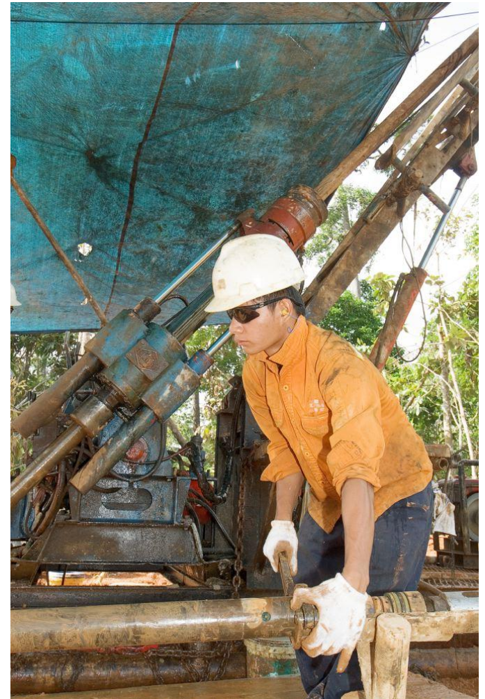
Diamond drilling, Bantian resource drillout
