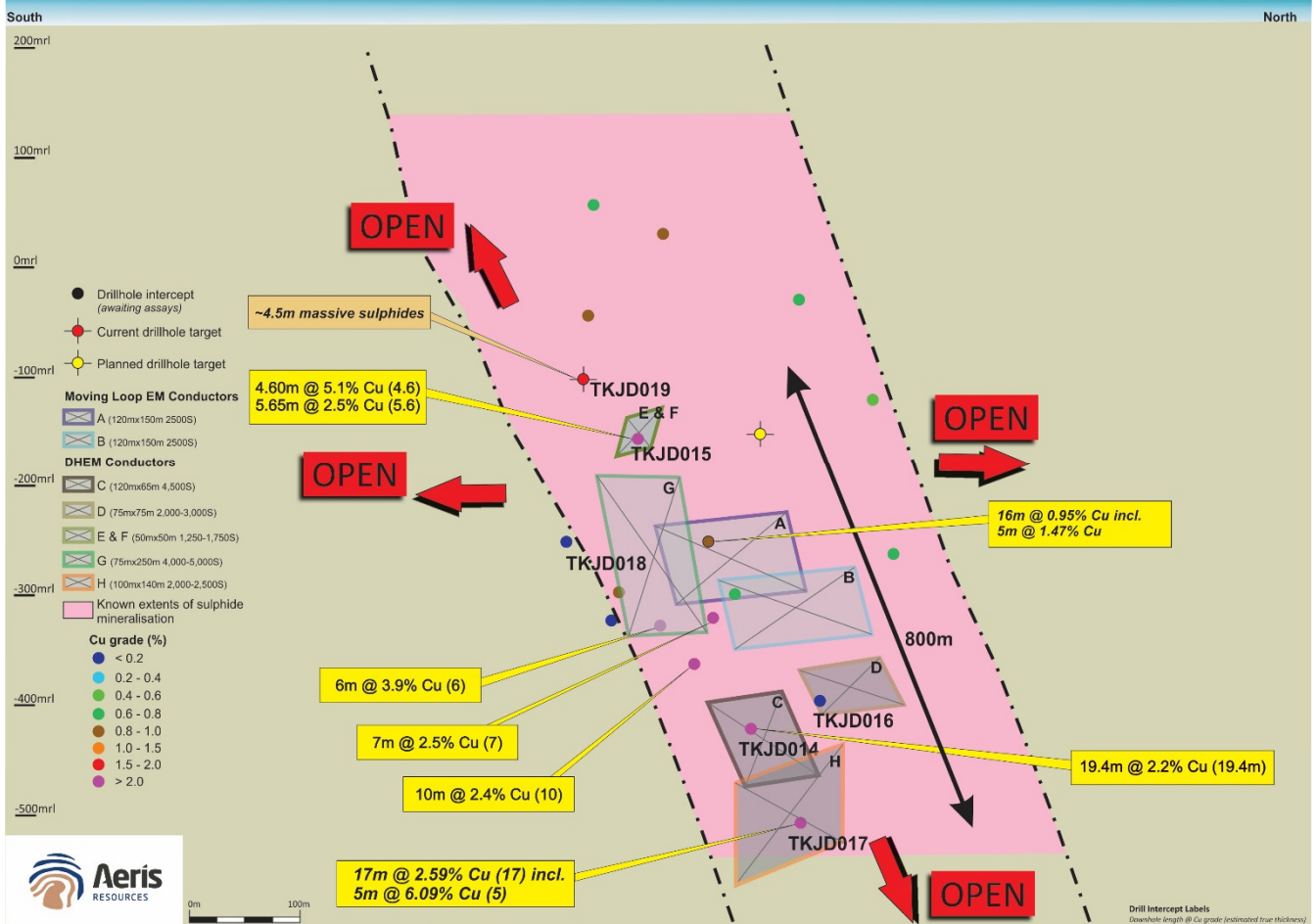
Figure 1 – Long section view of the interpreted Kurrajong mineralised envelope showing the location and copper grade from drillhole intersections through the sulphide deposit.
