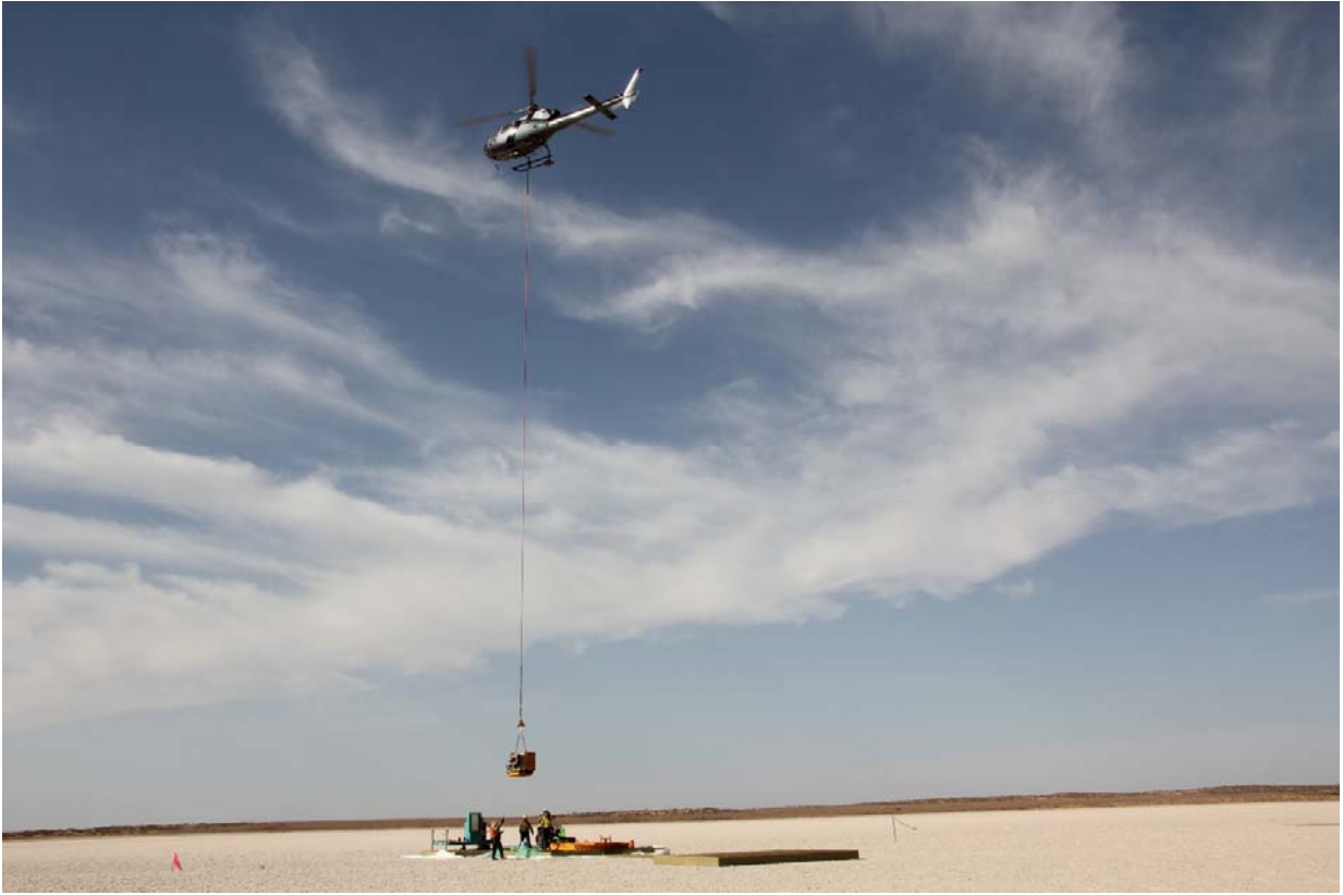
Figure 2: Helicopter transporting a section of the drill rig to the salt lake surface.
