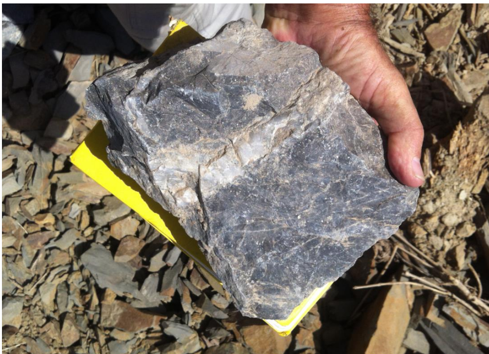
Plate 4: BouBou/Bourdala Permit – Bourdala/TD Artisanal Workings. Gold bearing quartz-carbonate vein in silicified-carbonate-sulphide altered meta-sediment.
