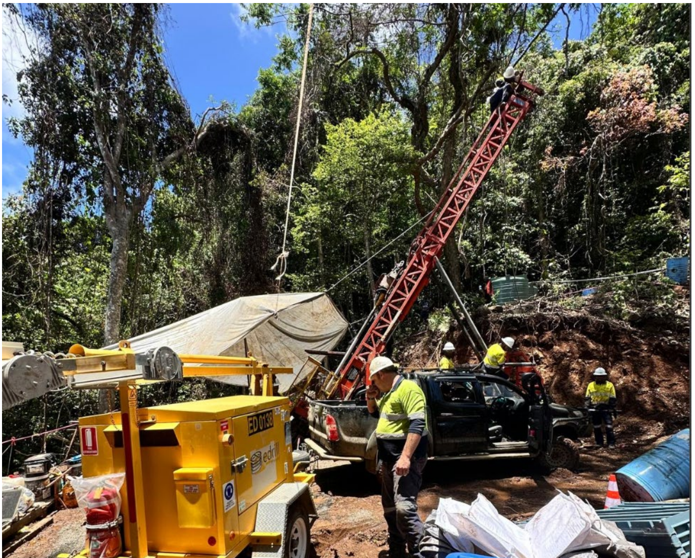
Figure 4 – Diamond drilling at Viani
