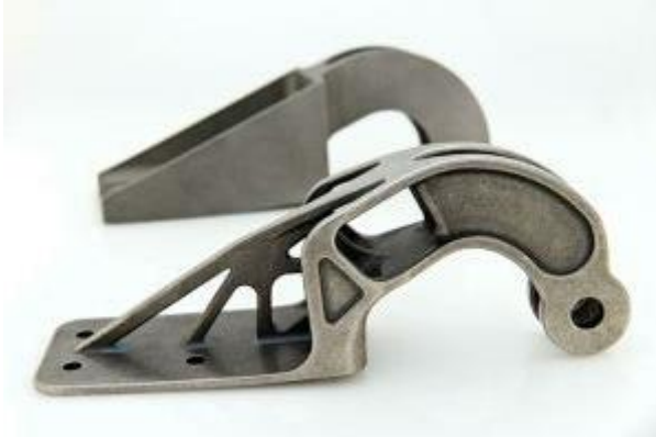
3D printed part (EADS-Airbus):
