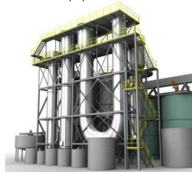
Resin-in-Pulp (cRIP) or Resin-in-Leach (cRIL)
