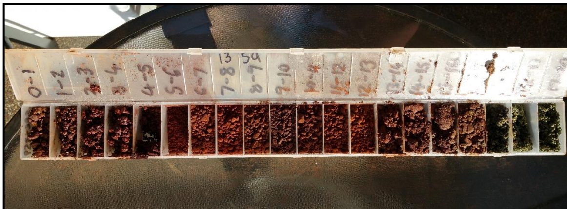
Figure 5: Hole SRC1359 chip tray showing 1m intervals through laterite profile, ending in basement ultramafic (green minerals on RHS of picture)
