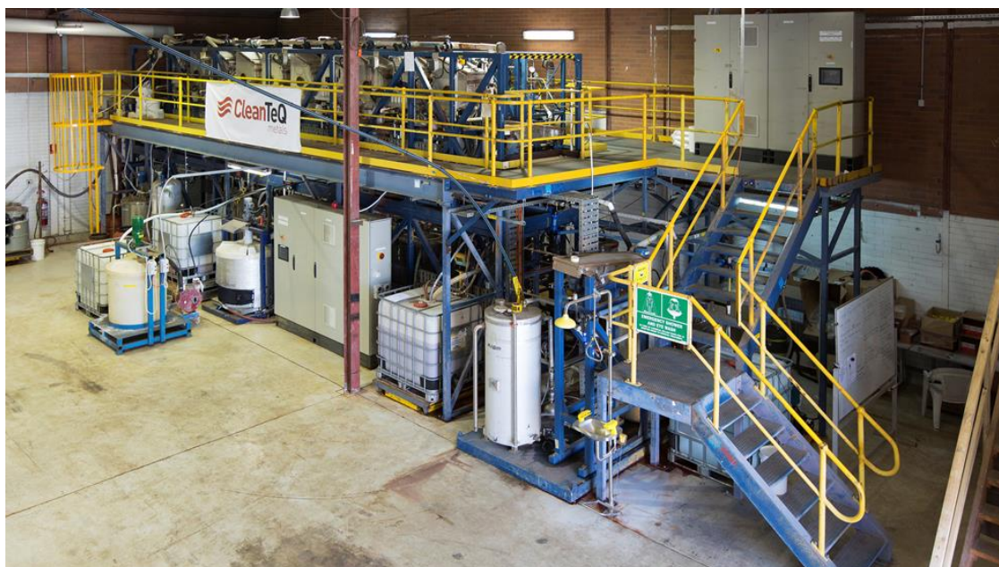
Figure 10: Clean TeQ's proprietary Resin-In-Pulp (cRIP) process demonstration plant, which can be used for production of NiSO 4 and CoSO 4 samples for customer testing
