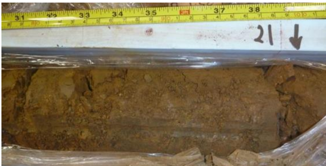
Figure 7-9: SDD016 20.85 m 6.6.2.3 GZ (Brown to Yellow, Extremely Weathered Goethite with Minor Mica)
