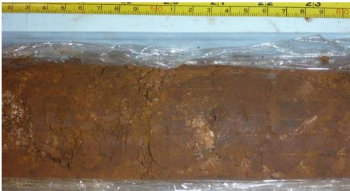
Figure 7-8: SDD014 7.5 m TZ (Brown to Orange Goethite-Clay with Minor Carbonate)
