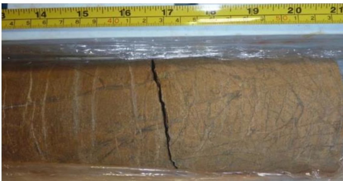
Figure 7-14: SDD021 40.42 m SAP (Hard, Brown to Grey Serpentinitic Saprock – Goethite-Serpentine-Carbonate)
