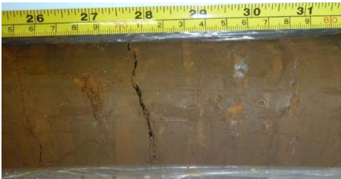
Figure 7-13: SDD014 30.75 m SGZ (Extremely Weathered Brown to Yellow Goethite-Clay, with White Patch of Quartz)
