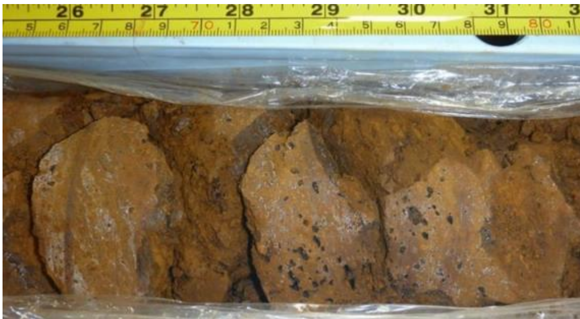
Figure 7-11: SDD021 31.73 m SGZ (Yellow to Brown, Silica-Goethite-Magnetite, with Clay Between Silicified Portions)
