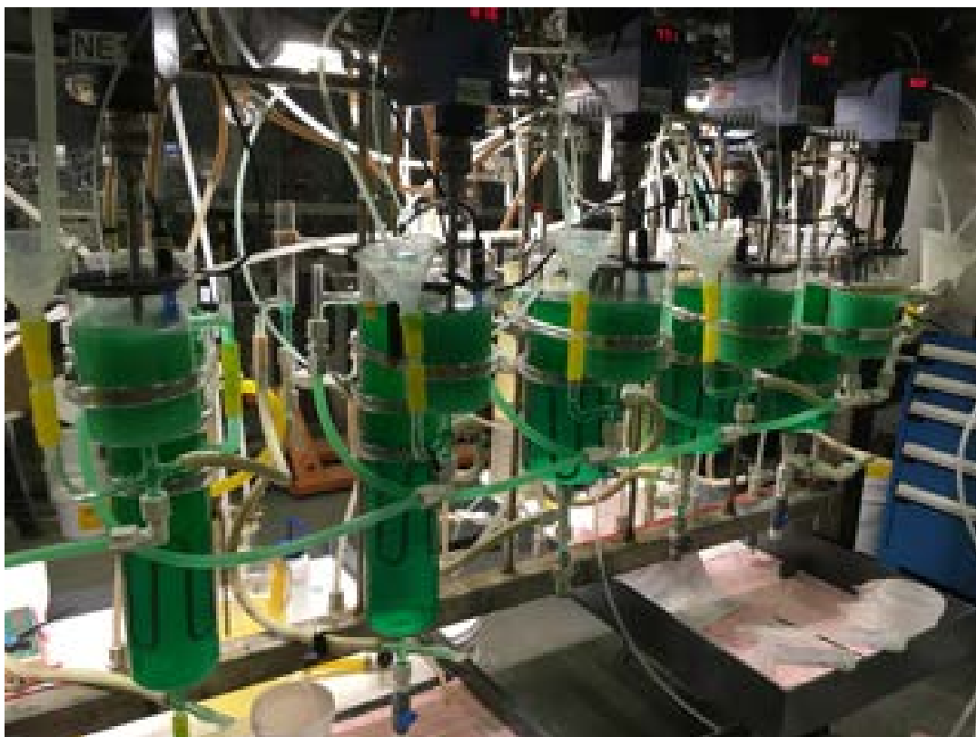
Figure 13-10: Nickel solvent extraction – 5-stage extraction circuit
