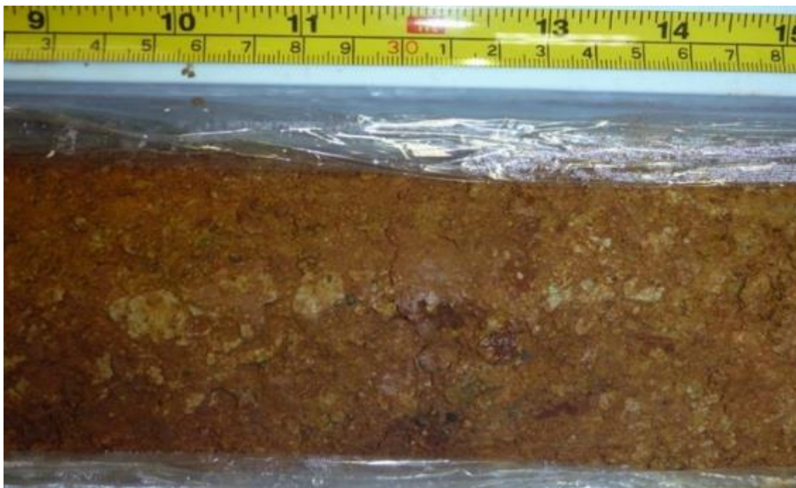
Figure 7-5: SDD015 2.30 m AV (Mottled Goethite-Clay With mm to cm Sub-Angular Gravel and Pisolites)
