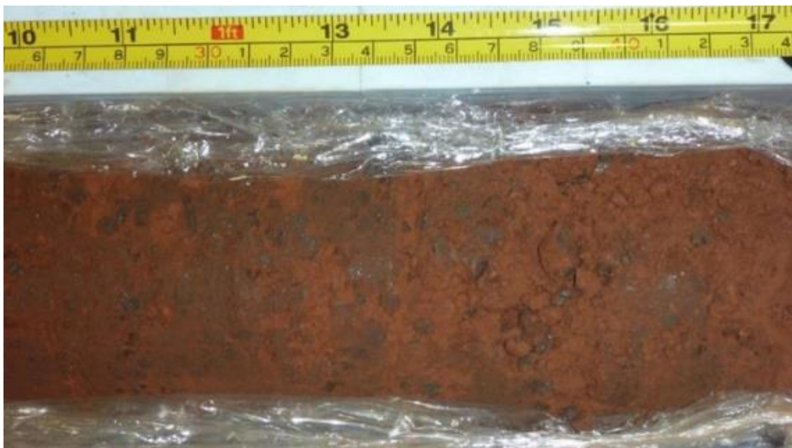
Figure 7-6: SDD021 4.30 m OVB (Red-Brown Pisolitic Gravel and Ironstone – Haematite-Clay-Maghaemite)
