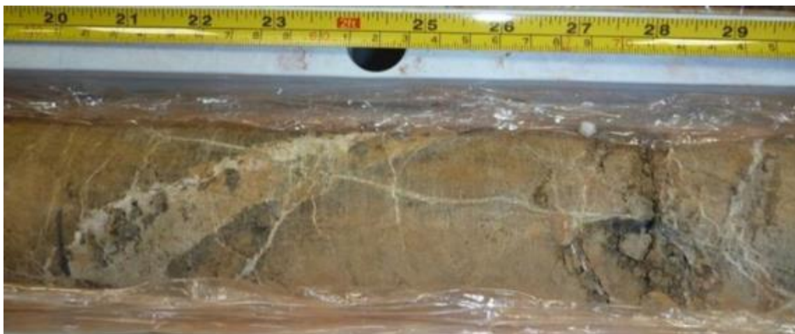
Figure 7-15: SDD016 43.60 m SAP (Goethite-Magnesite-Calcite, with Large Magnesite Vein and Narrow Calcite Veins)
