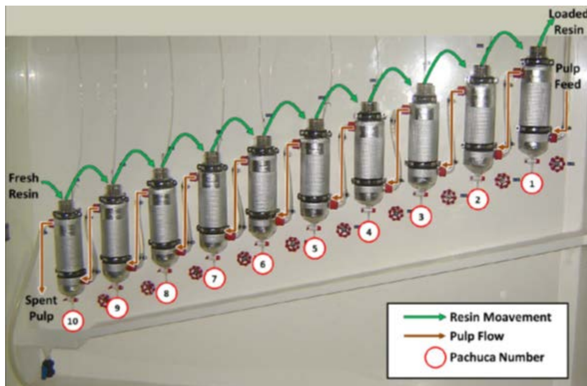
Figure 13-5: cRIP mini-pilot plant adsorption skid showing process stream movement
