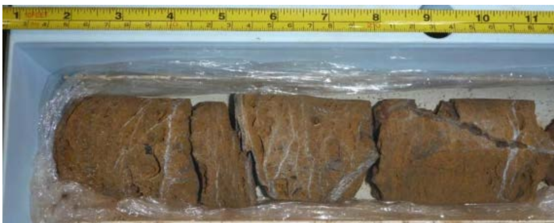
Figure 7-12: SDD015 37.2 m SGZ (Hard, Brown to White, Siliceous Goethite, with Narrow Quartz Veins)
