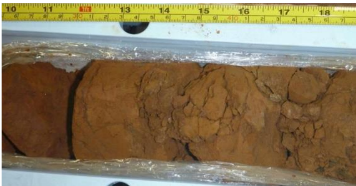
Figure 7-7: SDD020 5.37 m TZ (Medium-Hard, Brown to Red Goethite-Clay with Minor Haematite)
