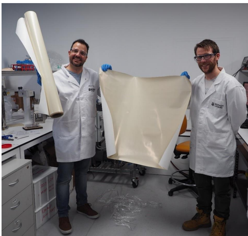
Figure 6 – Dr Sam Martin and Dr Sebastian Hernandez holding a graphene oxide membrane produced on an industrial-scale printer at the NematiQ facility in Notting Hill, Victoria
