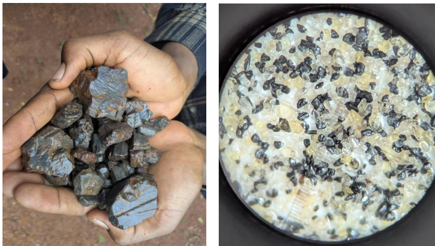
Figure 4: Rutile nuggets returned analysis of 98.4% TiO 2 (left); visible monazite and rutile in a panned Minta Est sample (right). The Company cautions that, with respect to any visual mineralisation indicators, visual observations and estimates of mineral abundance are uncertain in nature and should not be taken as a substitute or proxy for appropriate laboratory analysis. Visual estimates also potentially provide no information regarding impurities or deleterious physical properties relevant to valuations. Assay results from the drilling will be required to understand the grade and extent of mineralisation. Assay results are expected in Q4, 2026. Refer ASX announcement dated 2 July 2026 for further information.
