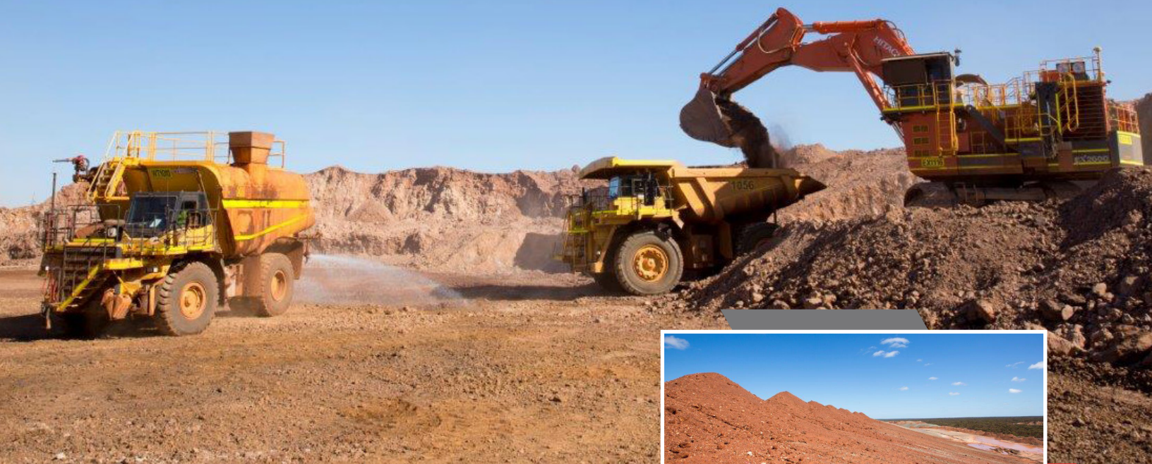
Image top: J4: Hitachi 2600 digger loading a Komatsu 1500 dump truck Image right: J4: New mine with progressive rehabilitation underway- topsoil ready to be pushed down
