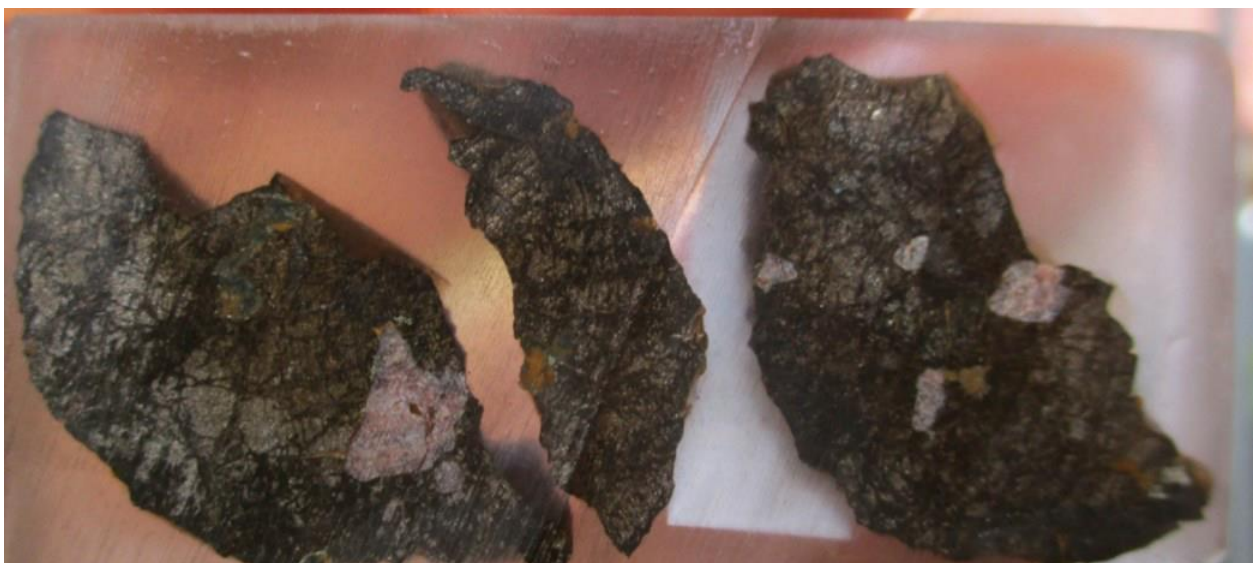
Figure 8: Sample 67 of appendix B ASX: PMM 01/12/2025 shows a pyrrhotite breccia with disseminated scheelite. This sample consists of quartz (grey-transparent) and scheelite (light orange to pink-coloured) clasts located throughout a pyrrhotite dominated matrix. Pyrrhotite in this sample is highly tarnished.
