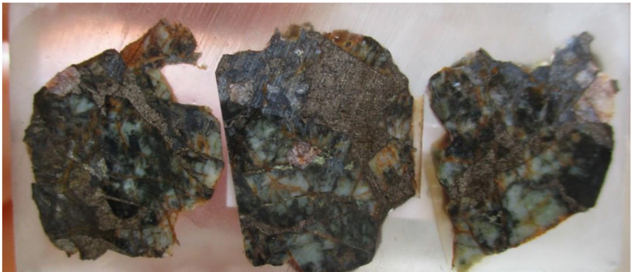
Figure 4: Sample 28, of appendix B ASX: PMM 01/12/2025 shows translucent to dark grey medium- to coarse-grained quartz set alongside pale to cream-colour medium-grained feldspar. The dark green to black flakes is interpreted as biotite and the light orange to pink colour blocky minerals are interpreted as scheelite. These Minerals are overprinted by a pyrrhotite dominated matrix with visible interspersed chalcopyrite.
