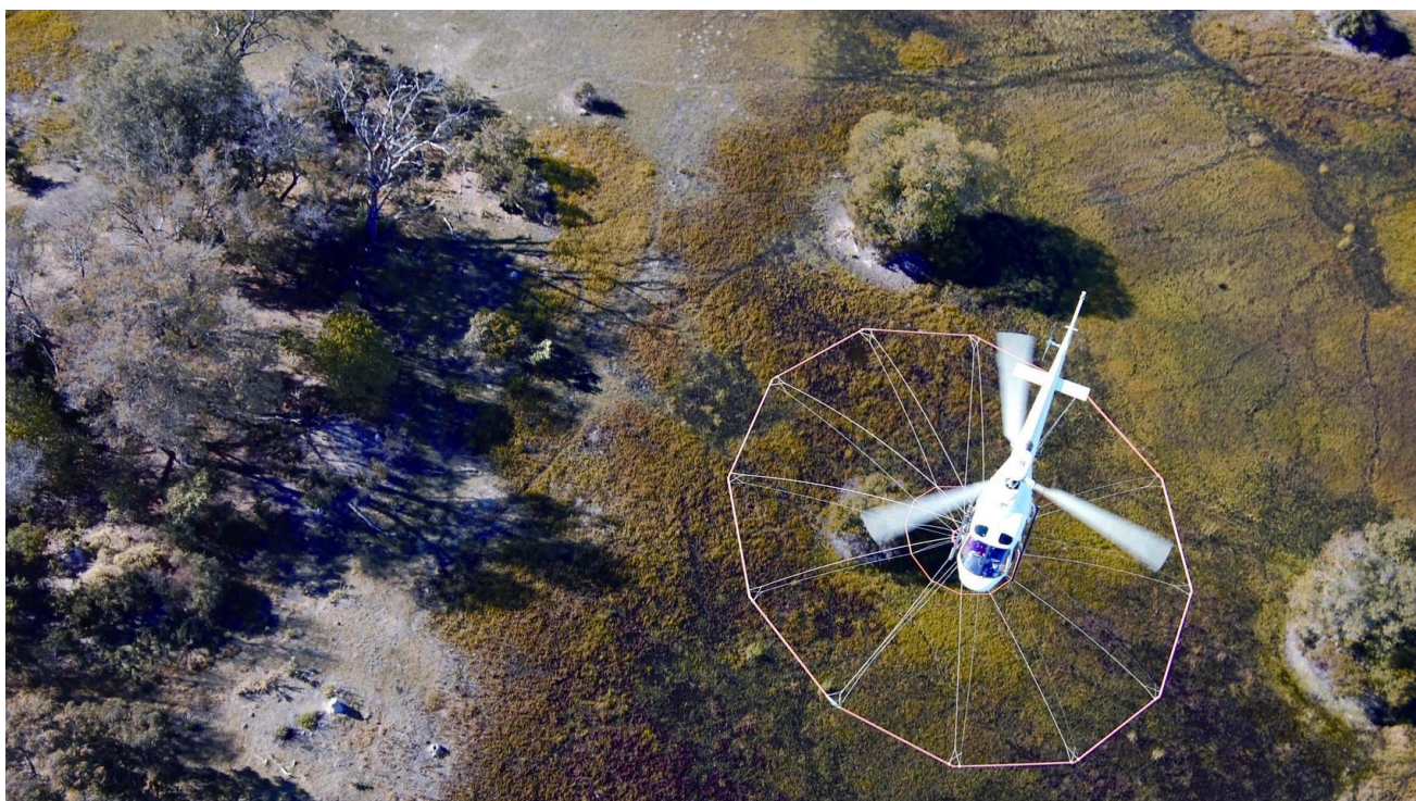
Figure 1: Example photo of airborne VTEM system used by GEOTECH to complete the VTEM survey at Springfield.
