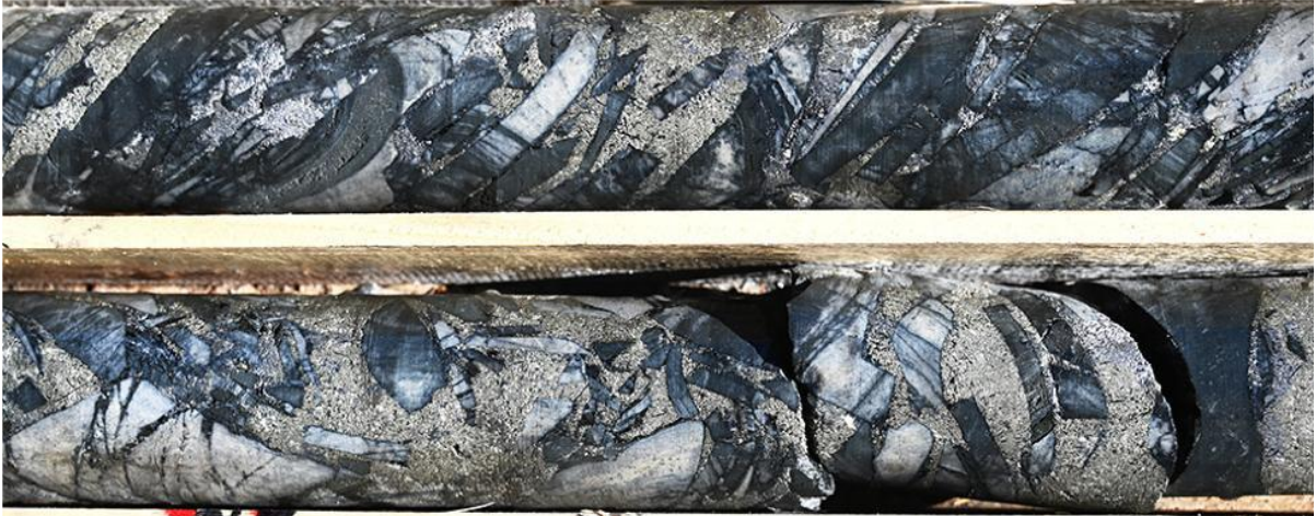
Figure 4: Gold-bearing breccia mineralisation: angular quartzite and siltstone clasts altered by sericite-silica, set within a pyrite-tourmaline-quartz-chalcopyrite matrix. SFDH-002, 75–76 m; from a 2 m interval averaging 5.6 g/t gold, 244 g/t silver, and 0.37% copper.
