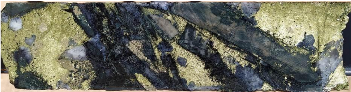
Figure 5: Angular, tourmalinised siltstone clasts supported in a chalcopyrite-tourmaline-quartz-pyrite matrix. SFDH-039, 452 m. From a 1 m sample averaging 2.3 g/t gold, 204 g/t silver, and 6.0% copper.
