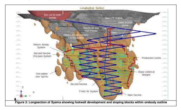
With a targeted ore production rate of 2.4Mtpa plus additional waste the mine haulage system was an important consideration for the project and crucial for sustaining projected cash flows. The incorporation of a second decline provides distinct advantages for efficient trucking with separation of equipment minimising congestion, allowing improved spatial layout for ore passes, better ventilation and a second means of egress.
