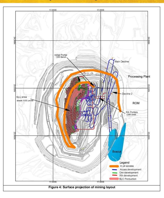
The proposed access locations for the fresh air and return airway portals have been located inside the pit which has schedule and cost advantages over shafts external to the pit which must be advanced through the surface oxide profile.
